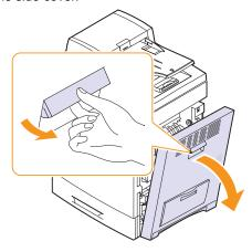
Remove the jammed paper, in the direction shown.
